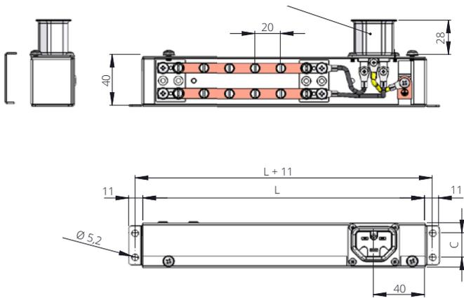
Casing with terminal strip, option: with plug 444.1 from 50 mm casing height
